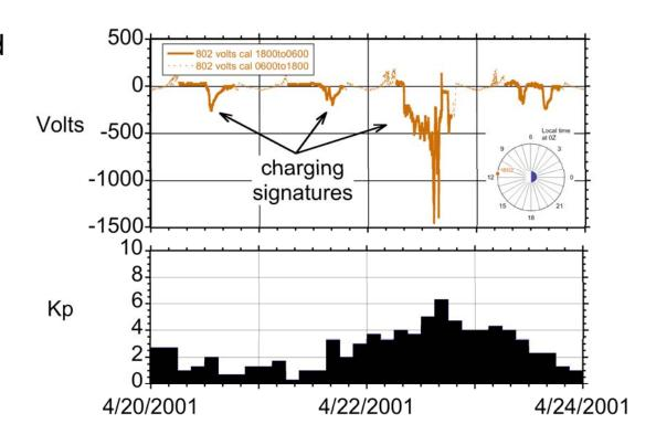
The Intelsat database benefits from very long time coverage, a clear response to plasmasheet electrons when the sensor is in shadow, and the ability to place a wide range of thresholds on the charging level
