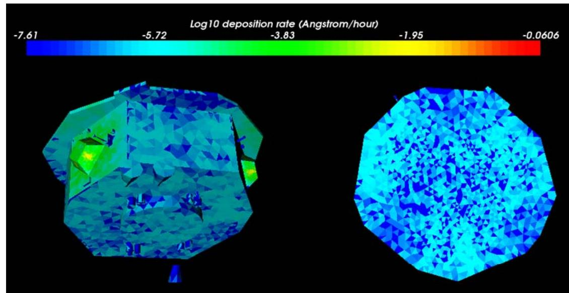
Cs contamination (0V) 99% efficiency
