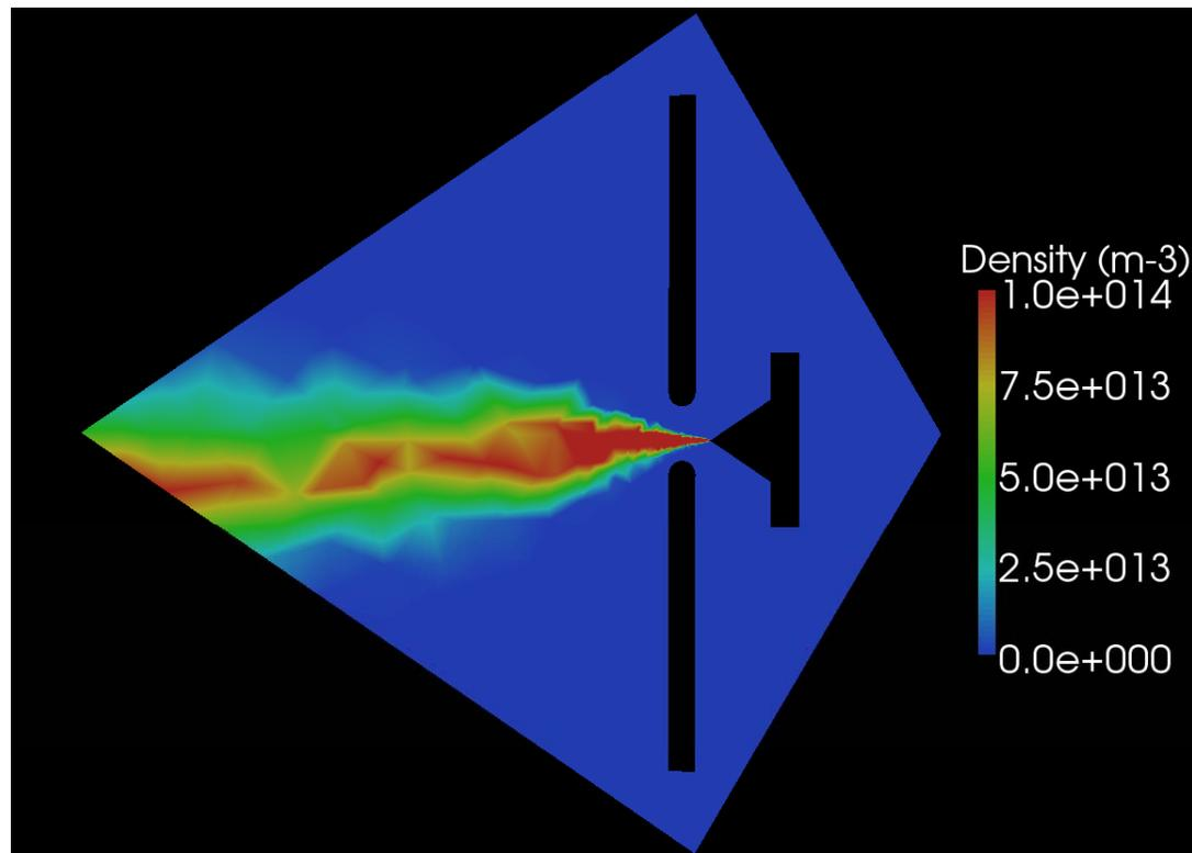
Emission with a displaced emitter (0.5mm down and 0.5mm away from accelerator)
