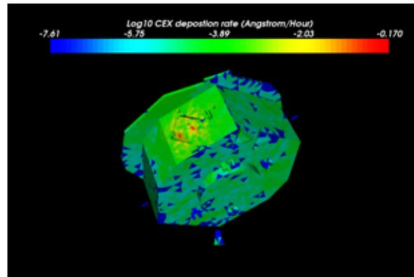
Cs contamination (0V and 150V spacecraft potential, 70% efficiency)
